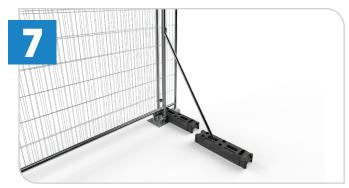
On the bolt-threaded side of the gate bar, secure the Std stabiliser and rubber fence foot on the inside of the site using an M12 nut and washer on the bolt-thread.
