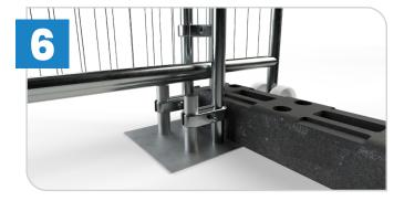
Using two HD Gripper Couplers, connect the gate base plate to the gate bar. Attach from the larger upright tubes to the gate bar on both sides of the gate.
